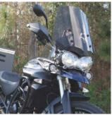
The wide range of position adjustments makes your windshield operate more aerodynamically by allowing air to flow underneath the screen to reduce vacuum effect - creating a far smoother airflow, virtually eliminating turbulence - and the difference in ride comfort is remarkable.
